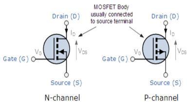
Enhancement-mode MOSFETs make excellent electronics switches due to their low "ON" resistance and extremely high "OFF" resistance as well as their infinitely high gate resistance. Enhancement-mode MOSFETs are used in integrated circuits to produce CMOS type *Logic Gates* and power switching circuits in the form of as PMOS (P-channel) and NMOS (N-channel) gates. CMOS actually stands for *Complementary MOS* meaning that the logic device has both PMOS and NMOS within its design.
