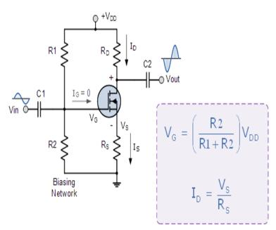
The DC biasing of this common source (CS) MOSFET amplifier circuit is virtually identical to the JFET amplifier. The MOSFET circuit is biased in class A mode by the voltage divider network formed by resistors R1 and R2. The AC input resistance is given as  $R_{\text{IN}}=R_{\text{G}}=1\text{M}\Omega.$
