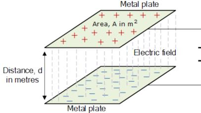
We have said previously that the capacitance of a parallel plate capacitor is proportional to the surface area A and inversely proportional to the distance, d between the two plates and this is true for <u>dielectric medium</u> of air. However, the capacitance value of a capacitor can be increased by inserting a solid medium in between the conductive plates which has a dielectric constant greater than that of air.
