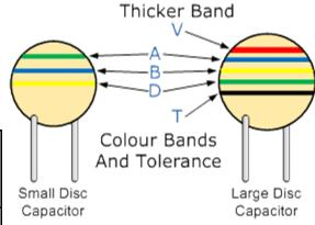
The **Capacitor Colour Code** system was used for many years on unpolarised polyester and mica molded capacitors. This system of colour coding is now obsolete but there are still many "old" capacitors around. Nowadays, small capacitors such as film or disk types conform to the BS1852 Standard and its new replacement, BS EN 60062, were the colors have been replaced by a letter or number coded system.
