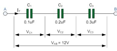
In the previous parallel circuit we saw that the total capacitance,  $C_T$  of the circuit was equal to the sum of all the individual capacitors added together. In a series connected circuit however, the total or equivalent capacitance  $C_T$  is calculated differently. The voltage drop across each capacitor will be different depending upon the values of the individual capacitances. Then by applying Kirchhoff's Voltage Law, (KVL) to the above circuit, we get:
