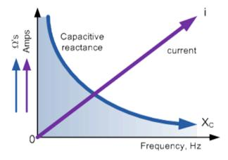
The capacitive reactance of the capacitor decreases as the frequency across it increases therefore capacitive reactance is inversely proportional to frequency.
