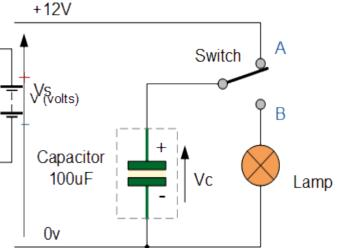
Assume that the capacitor is fully discharged and <u>the switch</u> connected to the capacitor has just been moved to position A. The voltage across the 100uf capacitor is zero at this point and a charging current ( i ) begins to flow charging up the capacitor until the voltage across the plates is equal to the 12v supply voltage. The charging current stops flowing and the capacitor is said to be "fully-charged ". Then, Vc = Vs = 12v.
