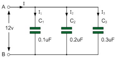
When capacitors are connected together in parallel the total or equivalent <u>capacitance</u>,  $C_T$  in the circuit is equal to the sum of all the individual capacitors added together. The currents flowing through each capacitor and as we saw in the previous tutorial are related to the voltage. Then by <u>applying *Kirchoff's Current Law*</u>, (KCL) to the above circuit, we have
