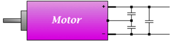
Figure 3. A three-capacitor filter. This is basically a combination of the one- and two-capacitor circuits.
