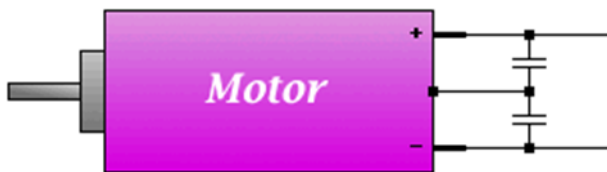
Figure 2. A two-capacitor filter. Each capacitor has one lead attached to a motor terminal, and the other lead attached to the case.
