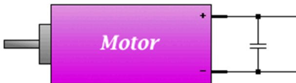
Figure 1. A single-capacitor filter. The capacitor is simply soldered across the motor terminals.
