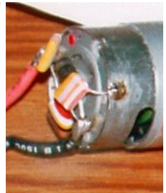
Photo 1. A typical three-capacitor filter installation on a ferrite motor. These particular capacitors are older style high-voltage ones; newer ones would be smaller. The black cylinder is the ESC's freewheeling diode.
