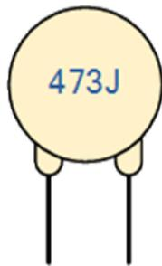
The capacitor on the left is of a ceramic disc type capacitor that has the code 473J printed onto its body. Then the 4 = 1<sup>st</sup> digit, the 7 = 2<sup>nd</sup> digit, the 3 is the multiplier in pico-Farads, pF and the letter J is the tolerance and this translates to:
