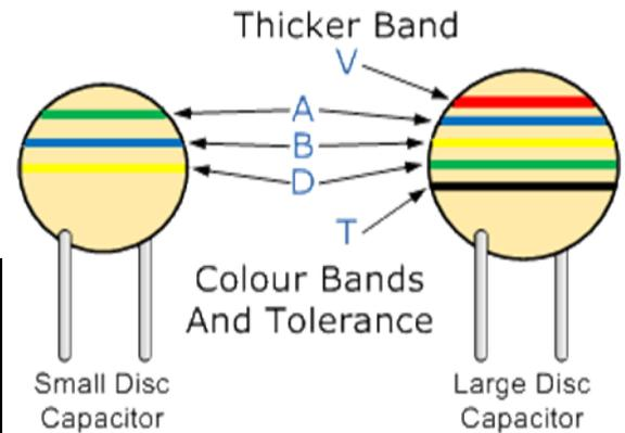
The **Capacitor Colour Code** system was used for many years on unpolarised polyester and mica molded capacitors. This system of colour coding is now obsolete but there are still many "old" capacitors around. Nowadays, small capacitors such as film or disk types conform to the BS1852 Standard and its new replacement, BS EN 60062, where the colors have been replaced by a letter or number coded system.
